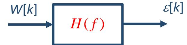
It is equivalent to a (narrowband) FIRST-ORDER IIR Filter operating at a rate  $1/T_0$
