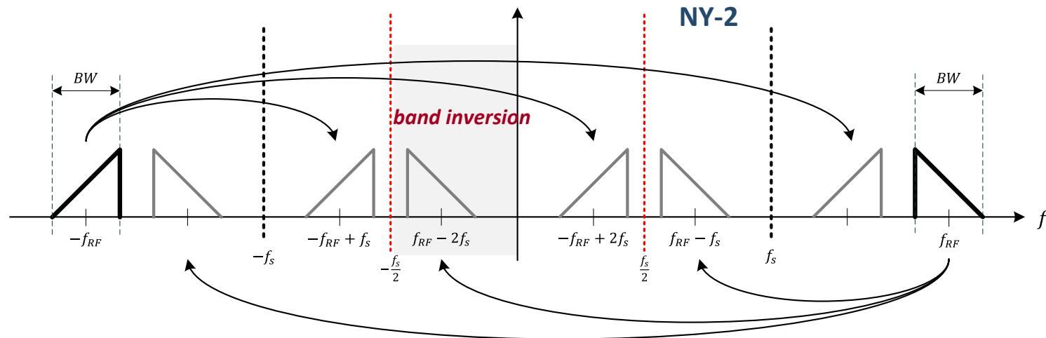
The resulting Digital IF is again derived from the relation  $f_{IF,D} = f_{RF} - mf_s$  where  $m$  is integer, but now it is in the *NEGATIVE HALF* of the digital bandwidth  $-f_s/2 \leq f < 0$
